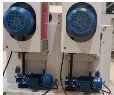
ELEVACION ELECTRICA/ ELECTRIC LIFTING
